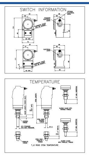
Details of Perseus Stainless steel switchcase with dual electrical connection options
